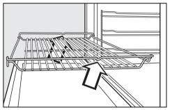
When pushing the rack back in, always ensure that the safety notches are at the rear of the oven (see illustration).
